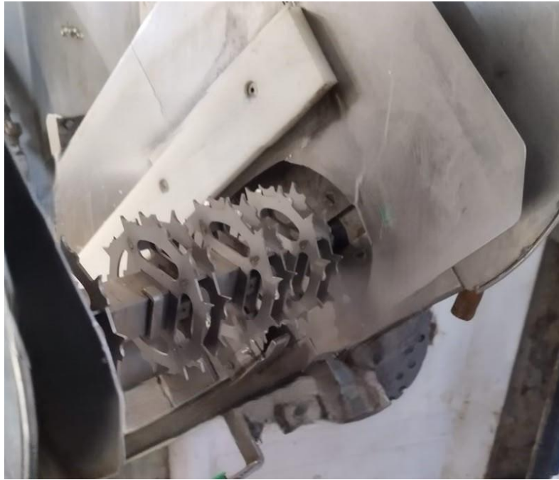
Sorting belt with plastic conveyor removed exposing the drive mechanism
