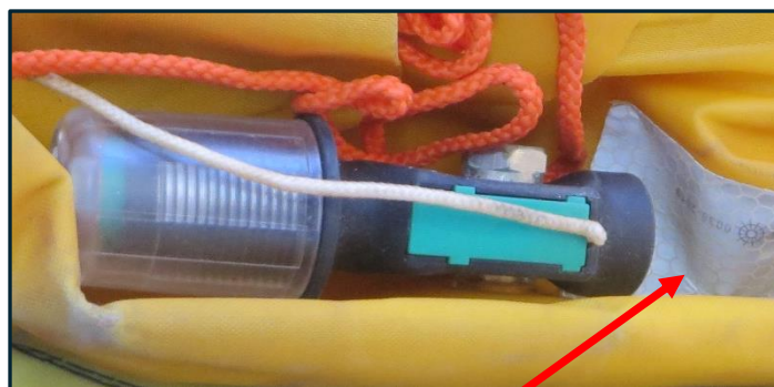
Figure 4: Co2 gas cylinder missing.
