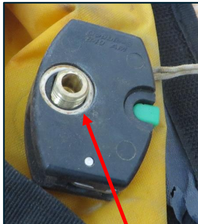
Figure 6: Securing nut missing.
