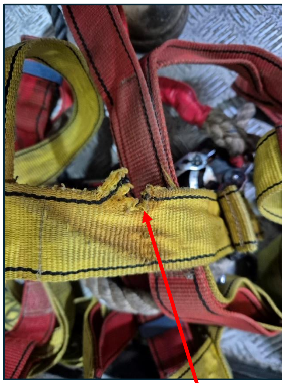
Figure 8: Safety harness showing rip in webbing.
