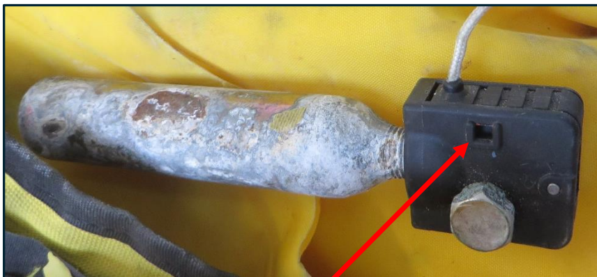
Figure 3: Release cord retention clip missing.
