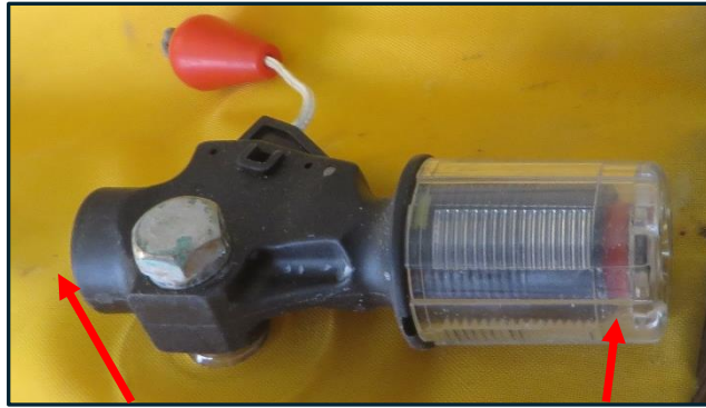
Figure 1: Automatic inflator activated and Co2 gas cylinder missing.
