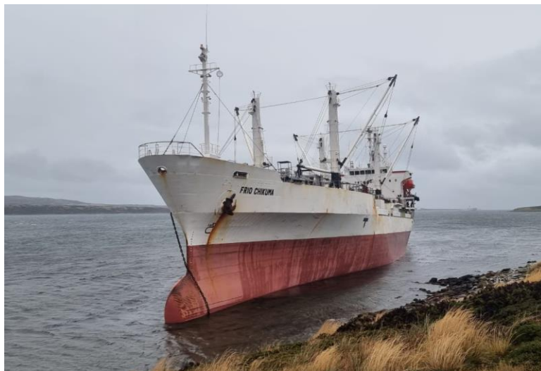
Figure 6: Starboard anchor chain caught under the bulbous bow – Photo courtesy of DNR, FIG
