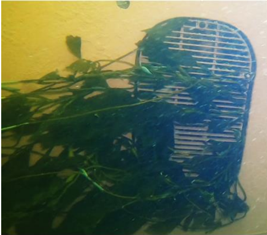
Figure 13: Starboard sea chest heavily fouled with Kelp
